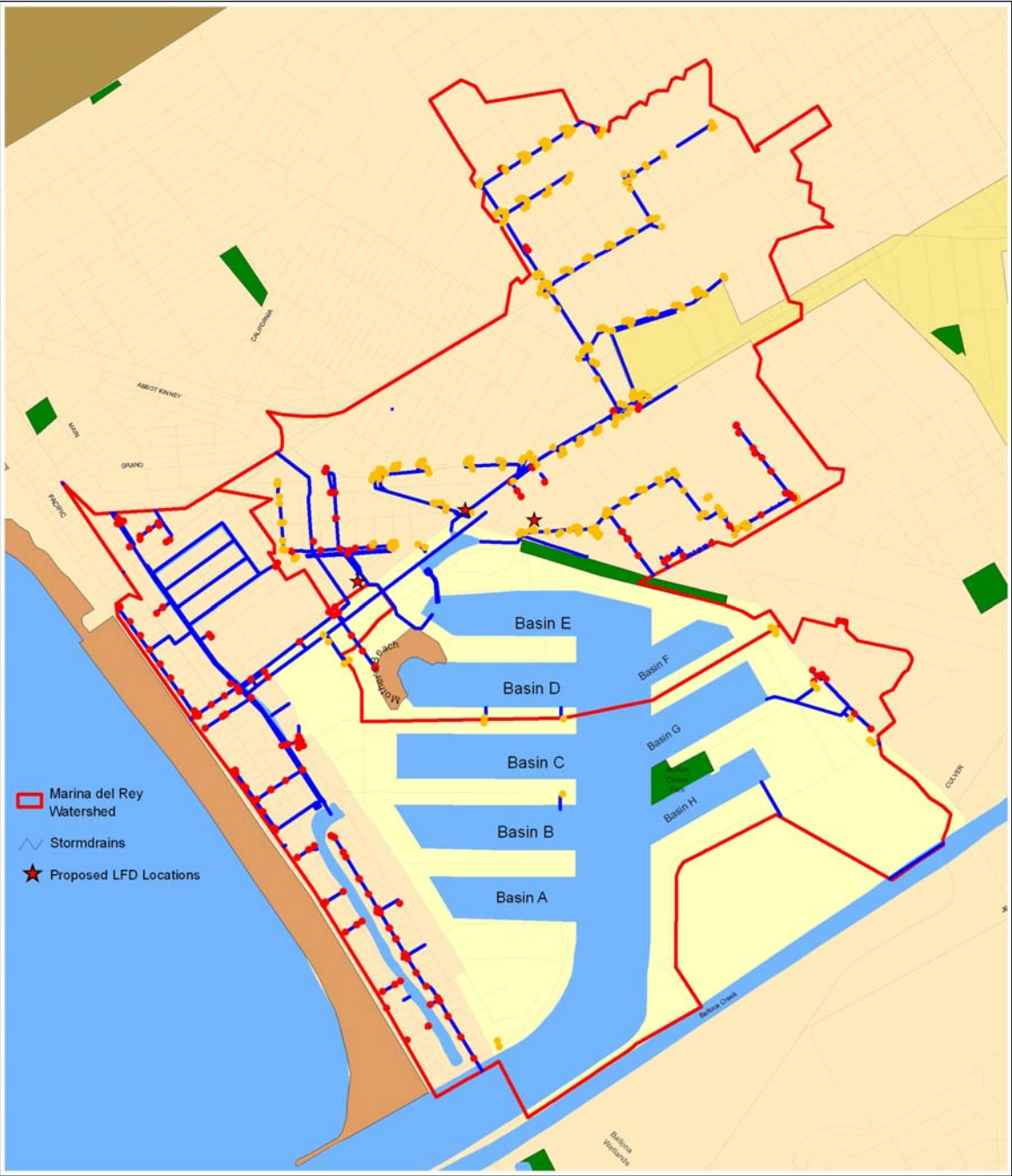
Figure 7-3 Proposed Locations of Low Flow Diversions for Marina del Rey Harbor Mothers Beach and Back Basins Bacteria TMDL
